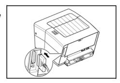
**NOTE:** Use a parallel printer cable that complies with IEEE 1284 standards. For optimum performance, install the printer close to the computer. The connection cable should be shielded and no longer than 3 meters (10 feet) long.
